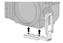
Slotted holes' ends have 1/4-20UNC thread as per the right illustration to use when removing pre-installed 1/4-20UNC Cap Screw (L12.5).
