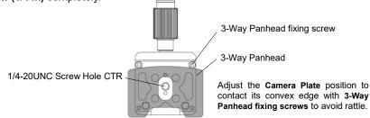
UW Tripod Hub: Shoe Base 1/4-20UNC  Screw the tripod screw (1/4 in) of the respective product into the 1/4-20UNC screw hole CTR on the bottom surface of the W50 Clamp Body to fasten two components.
