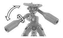
Loosening the Pan Handle enables to move the head back and forth.
