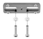
Put 1/4 Cap Screws (L) and <u>Tripod Screw Spacers (1.5mm thick) removed from the Main Base II</u> on the Panhead Adapter Base as shown on the above image.
