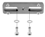
Put 1/4 Cap Screws (S) and M6 Washers on the Panhead Adapter Base as shown on the above image. (%Preinstalled when shipping)
