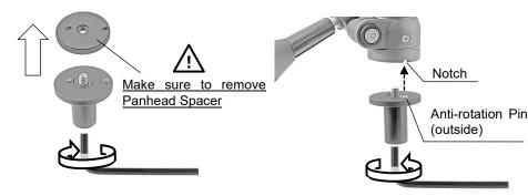
If the <u>Panhead Spacer</u> is attached on the Upper Elevator of the UW Tripod Hub, remove the spacer by using an Allen Wrench (3/16 in) which comes with the UW Tripod Hub. Apply grease on the threaded part of the pre-installed screw of the Upper Elevator (make sure to grease every time before using) then attach the Upper Elevator on the bottom of the Panhead so that the outer Anti-rotation Pin seats inside of the Notch of the Panhead. Then fasten them by using an Allen Wrench (3/16 in).
