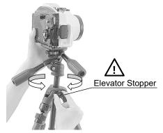
You can adjust the turning friction by the Elevator Stopper. Make sure to hold combined camera especially when loosening the Elevator Stopper to prevent abrupt falling of the Elevator.
