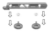
Remove 1/4 Tripod Screws and Tripod Screw Spacers from Main Base II (System Base II).
