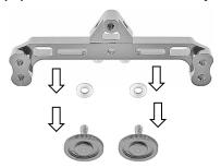
Remove 1/4 Tripod Screws and Tripod Screw Spacers from Grip Base M1.
