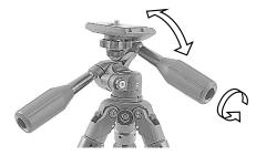
Loosening the Tilt Handle enables to adjust tilt angle.
