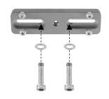
Put 1/4 Cap Screws (L) and M6 Washers on the Panhead Adapter Base as shown on the above image.
