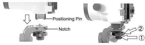
Put the 「Panhead Adapter Base」 on the Camera Plate so that Positioning Pins seat inside of notches without gap between the adapter surface and Camera Plate.
