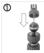
Attach the "Ball Adapter-Camera" to the arm ball and tighten it until it stops.
