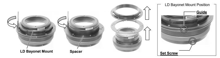
If you have any difficulty to unscrew M2x4 fixing screw(s), do not proceed any further. as you could damage fixing screw(s) and the original "M67 Screw Ring"/"LD Bayonet Mount" can not be separated from UCL-90/67 M67, UCL-90/67 LD. Please consult with your purchasing dealer for advice.
