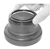
Then fasten them with supplied M2 x 7 fixing screws by using a precision philipps screwdriver #0 by making star pattern to tighten them evenly. <u>DO NOT</u> overtighten or tighten unevenly not to damage the lens itself.
