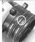
It is necessary to fill the space between UCL-165AD and housing port with water, so attach UCL-165AD underwater or partially unscrew the lens allowing inside air to escape then retighten.
