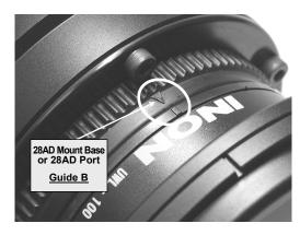
Attach the lens underwater or re-install underwater to escape air between housing lens port and UWL-100 28AD.
