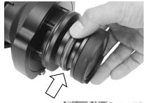
Then screw the Lock Ring M52 towards camera to lock lens position.
