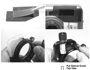
Remove Fiber Optics Fixing Dial, Fiber Optics Fixing Rubber and Cap Fixing Dial to dismount Optical Guide Cap WL and Optical Guide Mirror L. Then install those parts on the diffuser panel of AD Mount Base/M67 Mount Base in opposite procedure.
