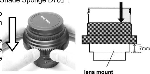
Make sure to press the Zoom Gear straightly against the lens barrel.
