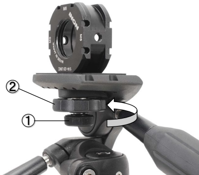
[UW 3-Way Panhead] Tighten ① then ②
