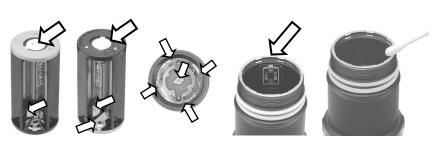
If above step fails to recover expected performance, conduct following maintenance on terminals (4 points) of the "LF1000-S Light Head".
