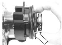
Then screw the [Lock Ring] towards camera to lock lens position.
