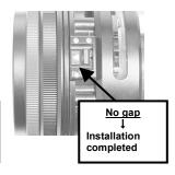
It is necessary to fill the space between UCL-67 LD and housing port with water, so attach UCL-67 LD underwater or partially unscrew the lens allowing inside air to escape then retighten.
