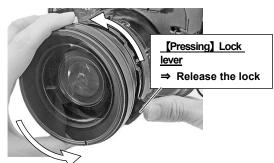
• Once submerged, remove the lens underwater and shake it well to drop trapped bubbles especially from the rear lens surface then install the lens on the XD Mount again following same procedure.
